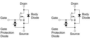
**Remark** The diode connected between the gate and source of the transistor serves as a protector against ESD. When this device actually used, an additional protection circuit is externally required if a voltage exceeding the rated voltage may be applied to this device.
