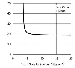
$R_{DS(on)}$  - Drain to Source On-state Resistance -  $m\Omega$
