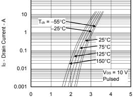
$V_{\mbox{\scriptsize GS}}$  - Gate to Source Voltage - V
